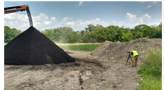
Finished compost is videotaped as it is deposited by a trommel screen at Cayuga Compost.
