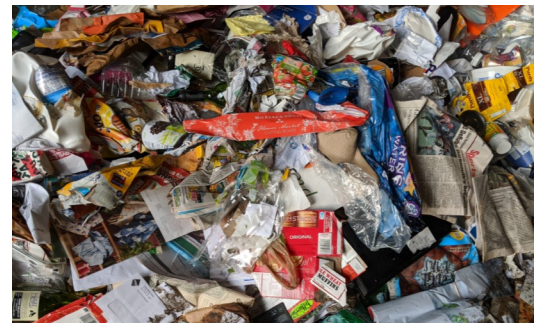
The recycling that arrives at the RSWC is often contaminated with plastic film, food, and styrofoam.
