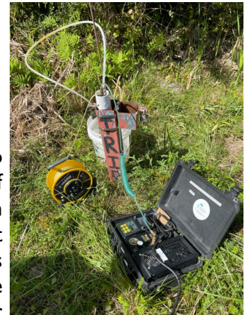
Testing equipment used to monitor the landfill wells.
